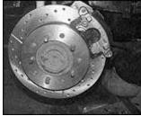
After attaching the new flexible brake lines to the hard line and bleeding the brakes, the instal- lation is complete. After heating up the brakes a few times, we noticed a considerable improvement in braking and reduced pedal effort, equating into a much more confident driving experience.
