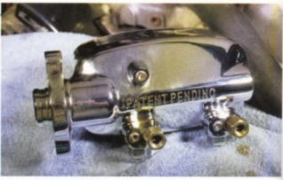
This view of the bottom of CPP's master cylinder shows a few things: bottom-fed ports, the adapter fittings installed in those ports, the redundant ports for front and rear (plugged), and the plugged port for the hydraulic brake light switch.
