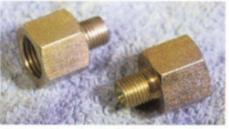
AutoZone will have plenty of these standard brake lines on the shelf. Nevertheless, if you want to reuse the old stock lines (which have 1/2-20 and 9/16-18 fittings, differentiating front from rear), this set of adapters (CPP PN MC-SF, \$15) will make it easy.
