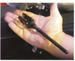
would need to be removed and swapped over to the new master. Note the fork where the pin holds the pushrod to the brake pedal.
