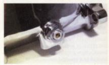
This is the adjustable proportioning valve in CPP's master cylinder. Note the concentric Allen screws—which separately control the max pressure to the rear circuit (innermost 1/8-inch Allen wrench), and the proportion of the rear circuit relative to the front circuit (1/4-inch Allen wrench). CPP provides detailed instructions with its master cylinder kit on maximizing your rear brake performance.
