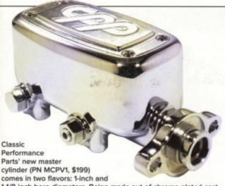
1 1/8-inch bore diameters. Being made out of chrome-plated cast aluminum, it's considerably lighter than most cast-iron master cylinders, and has a nice feature set, too. Key perks: built-in adjustable proportioning valve with adjustable max pressure, dual pressure ports for both circuits, a port for a hydraulic brake light switch, an extra reservoir lid for remote filling, and bottom-feeding ports for a cleaner appearance.
