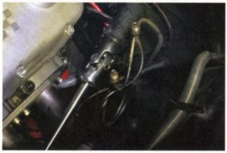
A previous owner of our '68 converted to disc brakes and didn't use a prop valve, so all we did was bend the brakes lines vertically to meet the bottom-feeding ports of the CPP master. If your Chevelle has a frame-mounted prop valve, you'll need to disconnect it, and run extension lines to the bottom of the CPP master. As we mentioned, the CPP master has a built-in adjustable prop valve, eliminating the need for the OE fixed-ratio prop valve.
