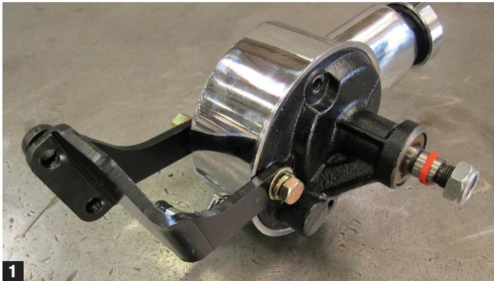
1. Loosely install the bracket onto the power steering pump and the engine using the threaded holes in the block nearest the timing cover, below the left-side freeze plug. (Figs 1, 2 & 3)
