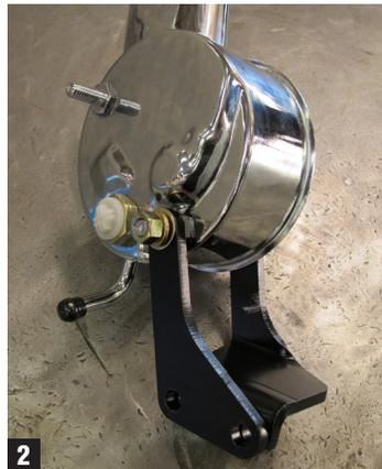
2. Loosely attach the adjusting arm bracket to the front of the pump and the engine. For "long" water pump applications, the dogleg in the bracket goes towards the engine; for "short" water pump applications, the dogleg points towards the pump. (Fig. 4)
