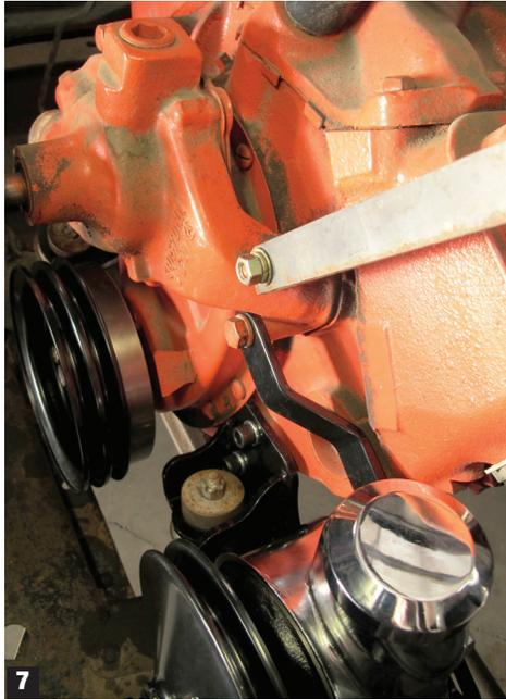
6. Verify the fit of your belts with the bracket positions; generally, a 15466 sized V-belt works best with a #CP38810 (PS pump), #CP38813 (dual-groove water pump), and #CP38811 crank pulley configuration. Tighten all bolts/nuts and adjust the belt tension as normal. (Fig. 8)
