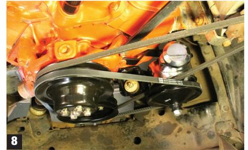
5. Typically, the adjusting arm will mount off the "lower" water pump bolt (especially to allow space for generator/alternator bracket arm); however, in some cases the upper location can be used. (Figs. 6-7)
