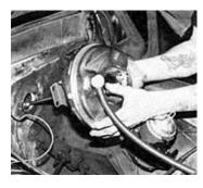
Now, slide the new power booster onto the firewall, lining up the bottom holes of the bracket with the two stock holes. Then mark the two upper holes of the mounting bracket to be drilled.
