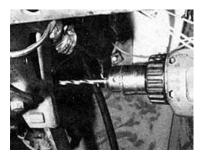
Mark and drill on the brake pedal arm where the rod end adjuster is to be attached while observing the action angle and clearance of the push rod.
