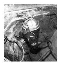
Here is what most 1962-'66 Chevy trucks with manual brakes will have, a single reservoir master cylinder hanging from the firewall.
