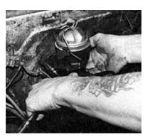
Begin by removing the stock master cylinder from the firewall. Do not remove the brake lines. Simply position the master cylinder slightly away from the area in which you are working.
