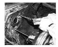
The firewall on these old trucks is very thick, so it's best to tap each hole mark with a center punch before drilling. Also, make sure that there are no obstructions such as loose wiring directly behind where you plan to drill.
