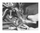
Once the spindle is exposed, and cleaned of all grease, it's the perfect time to check for any excessive wear in the wheel bearing. If so, the spindle must be replaced before this disc brake conversion can continue. Note simple Bolt-on of caliper bracket to the spindle's two existing mounting points. Also notice short spacer (arrow) used between spindle 's front boss and steering arm.
