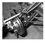
Since this was a prototype, we took measurements with the stock drum brakes, and then with the new discs, to see how much each wheel surface would move outward. Make that inward in this case, a substantial 1/8-inch.
