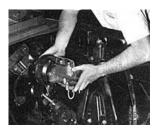
Talk about a sanitary installation of the Booster/master cylinder setup, it looks Better than a factory installation. Note neat wrap-around stainless steel hard line (optional) from proportioning valve to rear drum brakes. Complete disc brake kit part number is CPP-6467-DK.
