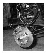
Here's the finished disc brake setup for the passenger-side wheel. In this instance, we got a bonus as we discovered that 14x6 American Racing Torq-Thrust "mag" wheels cleared the calipers. Now we can rely on stopping this '66 Nova much quicker and straighter than the previous factory drum setup.
