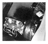
Jim Ries did his homework to come up with a booster/master/proportioning valve setup that would clear the Nova's shock fewer inner fender. As you can see, the plumbed assembly fits like a glove. The 7-inch Booster is coupled to a new 1-inch bore master cylinder, and a custom bracket supports a Delco proportioning valve, with all stainless lines.
