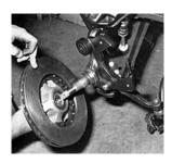
Rotors and hubs come unassembled, but it's an easy bolt-together situation here as the pieces are mated via a handful of 3/16-inch Allen bolts (10, to be exact). Again, Loc-Tite is a great idea, just to make sure. Assembled rotor/hub can now be fitted adequately greased Timken bearings/dust seal, then unit can be slipped onto spindle, followed by tightening of spindle nut over washer and outer wheel bearing.
