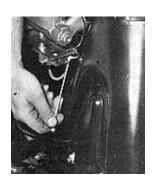
As you can see, it's a close fit between master cylinder assembly and inner fender, but it does clear. Also, fire hard line (shown being tightened with 3/8-inch wrench), that goes to driverside inner fender fitting, can still be removed.
