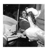
Before each caliper can be mounted, a center boss must be ground flush in order to clear the new caliper mounting bracket.
