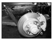
2. Our ice cream truck already has a Classic Performance Products disc brake conversion kit and is low enough to suit our tastes. It just needs to steer smoother and easier, and it will soon. Note the position of the front shock. We planned to relocate the top mount rearward for clearance.
