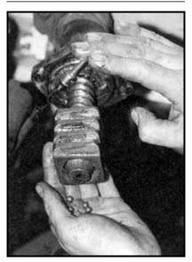
3. It was interesting to pull the old steering box off the end of the column to see how the small steel recirculating balls were packed in grease inside the box.
