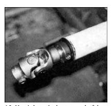
15. Here's how the bottom end of the column looks with the Teflon spacer located inside the column tubing. The steel inner shaft was now connected to a Borgeson universal unit and a locking collar was located in between to keep the Teflon spacer in place.
