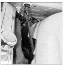
19. We used a section of steel D-shaft between two Borgeson universal joints to connect the original column with the Saginaw box. A little trimming of the inner fender panel was required to clear the D-shaft.
