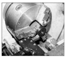
14. Just a little lathe work was needed to reduce the diameter of the Teflon spacer to match the inner diameter of the outer tube. We wanted a press-fit, so we checked it carefully to make sure it didn't get too small. Yeah, it would have been somewhat easier to install a more modern column, but we wanted to retain the original steering wheel and small-diameter column to keep a vintage appearance.
