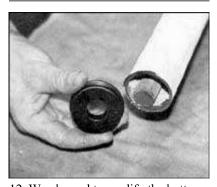
12. We planned to modify the bottom end of the original column by adding this Teflon spacer to the inside of the column housing and around the outside of the inner steering shaft. But first there were a couple of custom operations to be performed.
