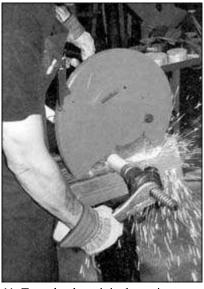
11. To make the original steering column work with the new Saginaw box, it was necessary to modify the bottom end of the column. The first order of business was to cut off the old, worn gear end.
