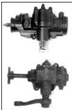
Here's the Saginaw 800 power steering box (top) compared to our
