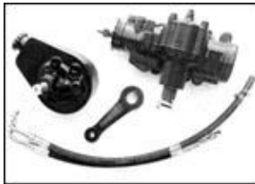
We went to Classic Performance Products to get the parts for the power steering conversion on our '65 Chevelle. The basic components included a rebuilt steering box and pump, a new Pitman arm, and new hoses.
