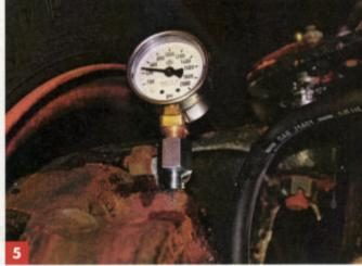
Moving to the front, and using a different adapter, the gauge was fitted to the calipers, each registering just under 500 psi. Hmm, more pressure at the rear than the front? No wonder I'm having trouble stopping this thing!
