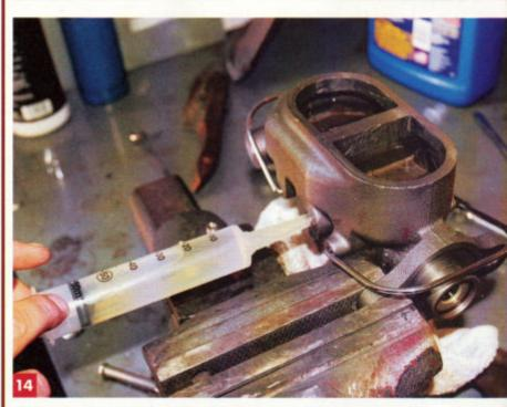
The bungs were removed individually and the large syringe from the kit was used to "back-bleed" the master cylinder through the outlet ports. A surprising amount of air was released back into the reservoir during this stage. The bungs were then refitted in order to install the master cylinder on the car.
