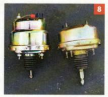
Here's the old (right) and the new (left). Both share the same mounting bolt pattern but the double diaphragm version is a littler longer. While this wouldn't be a problem in many cars, it will cause interference issues in my pickup. I temporarily unbolted the inner fender at the bottom for clearance
