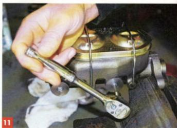
With the master cylinder clamped in a bench vise, the bungs were tightened in the outlet ports.
