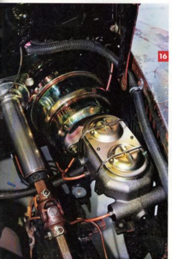
With the booster and master cylinder fitted, I again checked the pressure at each wheel; the rears still showed 650 psi and the fronts were up to 750 psi. It is recommends they should be 800 psi for disc brakes and 500 psi for rear drums, so the pickup's a lot closer than when I started, but not quite ideal. However, the brakes work much better now, and feel like those on a modern car.
