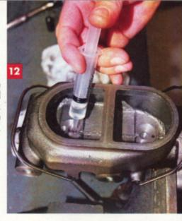
Using a rod to act as the booster pushrod, I slowly operated the master cylinder to release any air bubbles.
