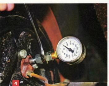
Installing the pressure gauge is as easy as removing the bleeder screw and fitting the gauge in its place with the correct-size threaded adapter. Starting at the rear, both left and right wheel cylinders showed 525 psi with the engine running and the brakes applied.
