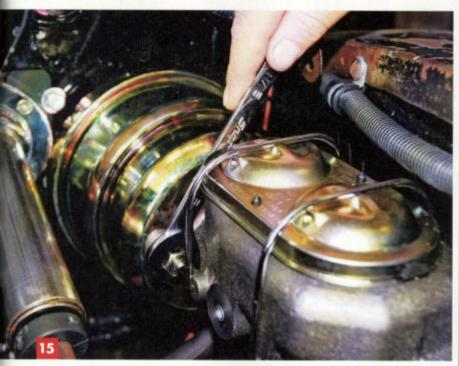
The master cylinder was then fitted to the booster, after checking the bore depth again. With permanent bungs in the left-side outlet ports, the brake lines were fitted to the right side one by one, each one left slightly loose and the pedal gently applied to bleed air. The whole system should be bled, but this sometimes can work, and did in this case.
