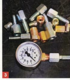
The kit includes a number of adapters to fit the pressure gauge, as well as blanking plugs and brass fittings to connect the gauge to junction points in the system if required. Here the gauge is fitted with the adapter for the GM calipers.
