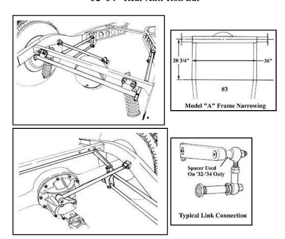
CPP's '32-34 rear anti-roll bar has been designed to bolt on to TCI '32-34 frames. This unit may be adapted to most other frames by installing a simi- lar tubular rear crossmember.
