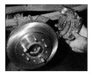
After temporarily securing the rotor to the axle with the wheel nuts, the caliper is installed. Make sure the bleeder valve is at the top.
