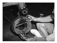
There are four bolts visible from either side which mount the backing plate to the axle flange. Remove all four and set the backing plate aside-forever.
