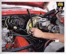
convert the 3/8-inch port to a 1/4inch port. CPP has a full selection of these plumbing adapters and fittings.
