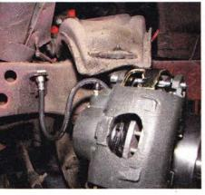
After all these procedures were done on the driver's side, Matt moved onto swapping out the hard brake lines. The lines that run from the master down to the front brakes are what we are going to replace since they need to be a bit bigger to feed the discs, and also because we are converting to power
