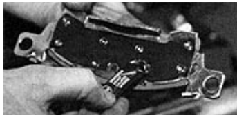
A socket is used to tap the cap home.
