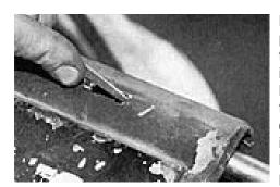
Since the cuts won't be perfect, a small file is used to remove the extra metal and form a smooth opening free of burrs.
