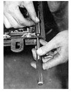
The first thing to do is remove the locking pin and spring by removing the plastic knob. Then, position the housing by centering it within the area of the upper tailgate lip. A center punch is then
