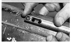
Check the position of the new holes by sliding the housing into the tailgate. Also check the holes by inserting the mounting screw through the housing and into the hole. You can see how the other two holes become the outer edges of the area needed to create the sliding knob gap.
