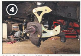
▲Now is the best time to install the caliper mounting bracket to the spindle. Using the supplied hardware, the caliper bracket mounts to the top of the spindle using a large bolt threaded into the spindle itself, and to the two lower mounting locations that also secure the steering arms. In the kit is a supplied washer that must be installed to make up for the added material of the caliper
