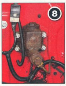
We then unbolted the factory manual brake master cylinder from the firewall via four bolts. Also. you need to slide out the pin holding the brake rod to the brake pedal itself. This requires getting under the dash and into the pedal assembly. This was made much more difficult due to the three-on-the-tree manual transmission linkages on the column. I was forced to hold the clutch pedal to the floor in order to remove the cotter pin and detatch the brake nod.
