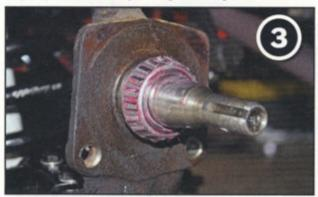
▲The installation begins by packing the rear bearing with grease and installing it on the spindle. Packing a bearing with grease is made much easier with a purpose-built grease packer. Make sure that both the outside of the roller bearings and inside are fully packed with grease, then place it on the spindle, and give it a roll. While rolling the bearing you should not feel any sort of resistance that can be caused by dirt or small rocks.
