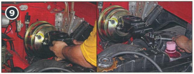
▲Next, we placed the 8-inch vacuum-assisted master cylinder assembly in place and bolted it down. The kit comes with both fine thread and coarse thread bolts to match your application. Make sure to take a look at the threads on the firewall and use the correct set of bolts. Tightening them into place takes some time, as one will tightenen, "loosening" the rest. Once you have them tightened, take one more lap around the four bolts just to make sure.
