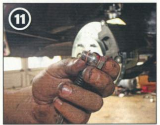
At this point, we could start working on the brake lines. The supplied flexible lines connect the calipers to the frame and allow for the range of motion in the steering wheel. They connect to the caliper using a banjo bolt that consists of a hole to allow for fluid movement internally. The fluid is then transferred to the braided brake lines' slotted ring, which seals itself and makes a leak-free connection.
