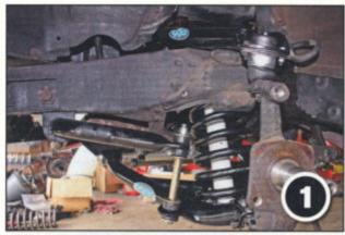
We started our installation with a bare spindle. At this point, we had our complete front suspension kit from CPP on the car and ready for the alignment rack. This kit re-uses the factory spindle and drops the front end with a set of shorter springs. We made sure to clean all of the mating surfaces of the factory spindle as they had accrued over 50 years of grease and grime.
