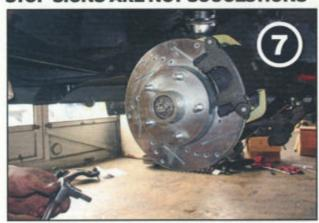
At this point, the main hardware of our disc brake assembly is complete. The pads and rotors can be replaced at the local parts store, and we have made leaps and bounds over our factory drum brakes. These 10.8-inch rotors will accept a 15-inch wheel and we left the Rallys on since they look so sweet.
