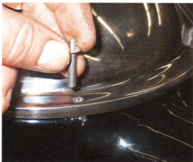
Special rivets were used to secure the cover. They are expanded and locked in place by driving in the center pins with a hammer and punch.
