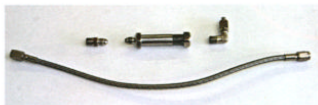
We used through-the-frame fittings to plumb the brake system. They, along with fittings, braided flex hoses, and line clamps, came from Kugel's.
