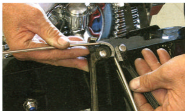
It's hard to make smooth, consistent turns in brake lines without a bender. They're inexpensive and will usually pay for themselves when compared to the tubing that's ruined trying to bend it by hand.
