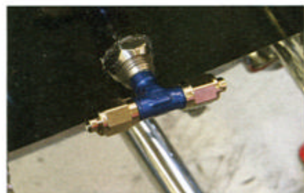
The left front through-the-frame fitting has been installed here. We used stainless lines with AN fittings, which require 37-degree flares.
