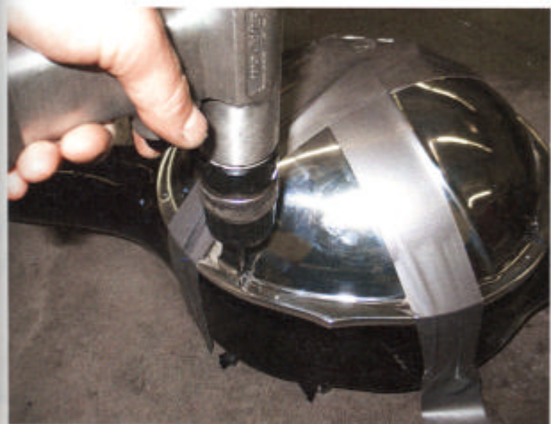
Duct tape was used to secure the cover while the silicone set. Then, using the holes in the cover as a guide, the housing was drilled for the special fasteners.
