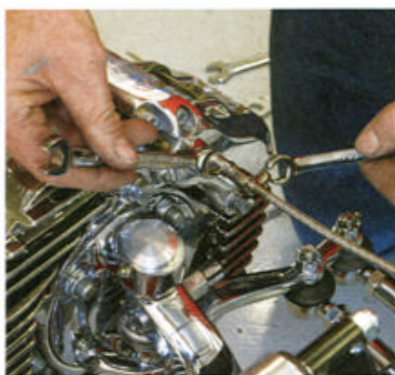
We used through-the-frame fittings to plumb the brake system. They, along with fittings, braided flex hoses, and line clamps, came from Kugel's.
