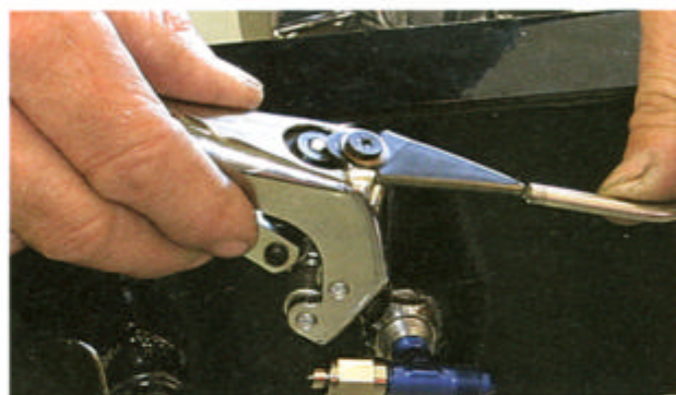
After brake line tubing is cut to length, always deburr the tubing before flaring. Even the smallest burr may cause the flare to split.
