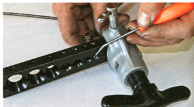
With most tools, the tubing should be flush with the outer edge before it's flared. Stainless line uses a single flare with a ferrule inside the nut to reinforce it.
