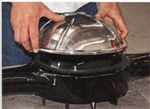
We installed a Pete & Jake's aluminum cover to give the new 9-inch housing from John's Industries a different look. After grinding away any rough spots, silicone was applied to the lip of the cover and it was pressed in place.
