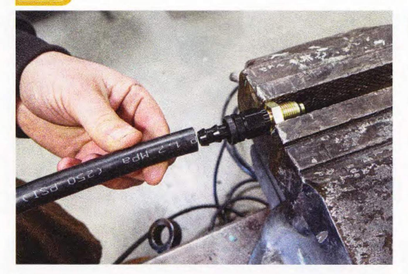
We started from the tank and worked our way forward to the engine. The supplied AN fittings are PTC (push to connect) and can be a real bear to properly seat the high-pressure hose completely onto the double-barbed fittings. (Use of heat as well as the suggested lubricant will help.)
