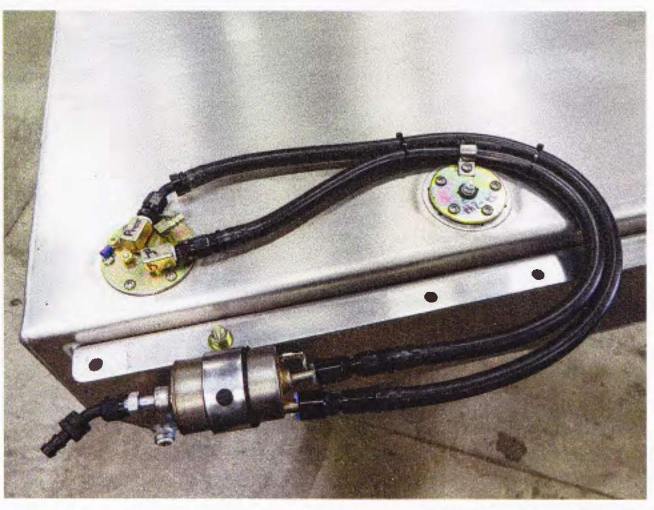
It was decided to mount the fuel filter directly to the rear mounting edge of the tank, and to illustrate how the dead-head return-style system was plumbed to this point, we dropped the tank back down.
