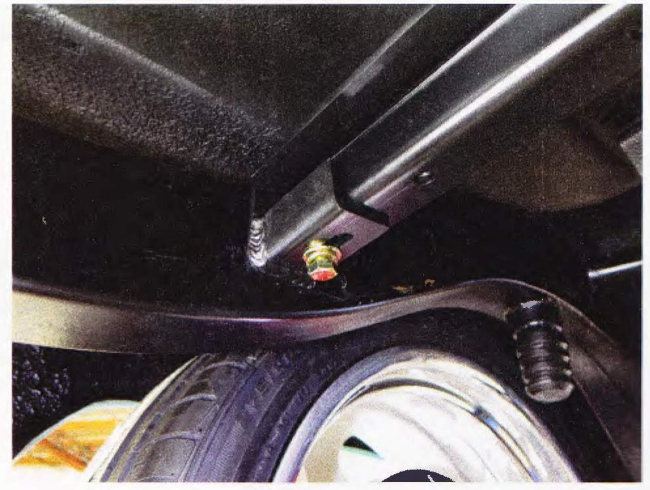
11 12 The forward crossmember features bolt-on framerail brackets, which can also be welded (which we will ultimately do), that are adjustable to accommodate both styles of '55-'57 Chevy 'rails—one piece (shown) or the welded two piece.
