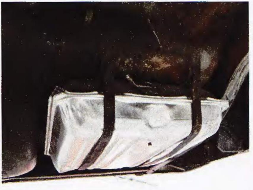
Here's what we'll be replacing: the stock '55 Chevy 12-gallon two-piece pinch-welded gas tank—with an over double the capacity fabricated-aluminum tank from Classic Performance Products. (Granted, at this stage we already got rid of that real-estate-robbing
