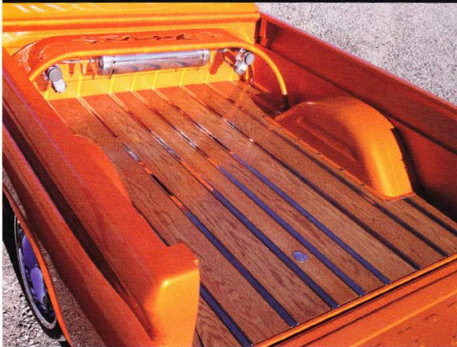
TOM'S C-10 SPORTS PLENTY OF EYE CANDY IN THE BED, WITH CUSTOM TOUCHES SUCH AS AN OAK FLOOR WITH STAINLESS STRIPS, A STAINLESS FUEL FILLER CAP AND A FABRICATED TUBULAR AIR MANAGEMENT MOUNT ON WHICH HANGS A POLISHED AIR TANK AND TWIN VICI AIR COMPRESSORS.
