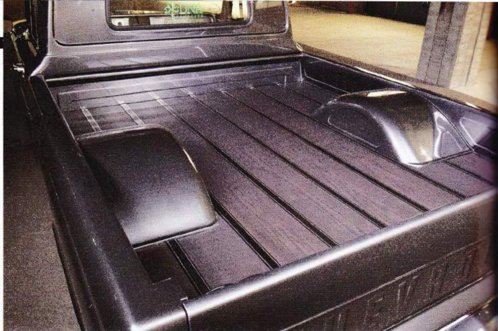
THE CUSTOM BED FLOOR WAS CRAFTED FROM OAK PLANKS AND CNC-MACHINED BILLET STRINGERS.
