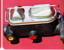
Prior to the 1967 model year, U.S. vehicles had single hydraulic braking systems with one master cylinder (above) tied to all four brakes. Dual braking systems (front and rear) became federally mandated beginning with the 1967 model year, and this is the only braking system to have even if you're building a stocker.
