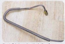
Classic Tube's pre-bent brake lines for rear axles have this anti-chafe coil to protect lines from road debris. You can specify the use of anti-chafe when you're ordering custom prebent lines.
