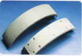
The age old debate addressing riveted versus bonded brake shoes continues to resonate, but in the end it boils down to what you want your brakes to do. Riveted linings carry heat away better than bonded; whereas, bonded linings provide more friction surface area.
