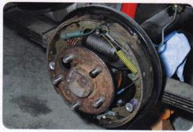
Rear drum brakes can be excellent performers given good preventative maintenance. With each and every brake job must come all new parts including drums, linings, hardware and wheel cylinders for optimum performance. When you turn brake drums and reuse them, you increase shoe and pedal travel, which is why it's suggested that you install new drums.
