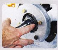
Absolutely never do this. Grease doesn't belong between the bearing and axle because the bearing race must remain stationary and secured to the axle spindle. We see this all of the time with the logic being corrosion prevention or lubrication; however, the bearing race/hub is not supposed to rotate.
