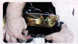
A dual brake system offers the greatest measure of brake safety because you still have brakes should the front or rear system fail. Regardless of whether you're building a stocker or a resto-mod, you must have a dual braking system with a proportioning valve for optimum pressure distribution and brake control.
