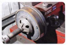
Brake drums are turned and machined all of the time. Machining limits are always cast into the drum. It's strongly suggested you replace the drums rather than turn them to keep pedal travel conservative.
