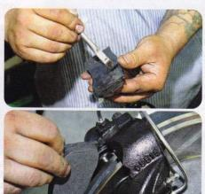
Brake pads should get noise reduction grease between the pad and caliper, which quiets brake operation and eliminates binding. Make sure rotors and friction surfaces are hospital clean before pads are installed. Clean rotors with a high-evap' solvent, like brake cleaner or lacquer thinner, and allow them to dry before pad installation.
