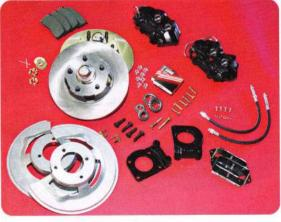
Stainless Steel Brakes Corporation offers a wide variety of disc brake packages from one- and two-piston iron caliper budget kits to high-end, large-disc jumbo jet binders. You can get into a budget front disc brake conversion kit for around \$1,000 and achieve excellent stopping power. Remember, anything beats fourwheel, non-power drum brakes. It's an investment in your own safety.
