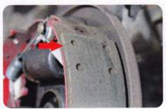
Brake linings crack from excessive heat and even high water, which thermal-shocks the linings, causing them to crack from a sudden change in temperature. When linings crack they must be replaced.
