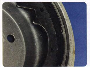
When you reline, check the lining-to-drum relationship and ascertain fitment. In the good old days, repair shops used to arc brake shoes for solid drum fitment. Those days are gone, but it's up to you to examine shoe-to-drum contact prior to assembly.
