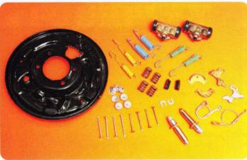
New brake backing plates and complete hardware kits are available from Summit Racing Equipment. You may also recondition existing back plates by welding in a rise at shoe contact points and grinding them flush to improve the shoe's relationship with the backing plate. Use white grease at these contact points to reduce wear. Don't overdo the grease.
