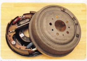
Rear drum brakes can be excellent performers given good preventative maintenance. With each and every brake job must come all new parts including drums, linings, hardware and wheel cylinders for optimum performance. When you turn brake drums and reuse them, you increase shoe and pedal travel, which is why it's suggested that you install new drums.
