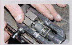
This is one type of flaring tool for the home garage fanatic. The Mastercool universal hydraulic flaring tool (P/N 71475) from Eastwood yields a precision fit and a perfect flare because it keeps the line centered on the flaring head. The Eastwood Company has a variety of brake line flaring tools hinged to your budget. Remember, you get what you pay for. Opt for higher ground and get better results.
