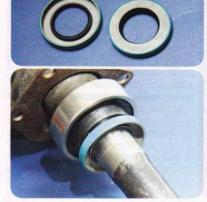
There are two basic types of axle seals: with a garter spring and without, Seals fitted with garter springs have to be handled carefully. Pack the spring cavity with wheel bearing grease, which keeps the spring secure while you're driving the seal in. Otherwise, the spring pops off and you will have leakage. Lubricate the seal lip generously to ensure a happy marriage with the spindle or axle shaft.
