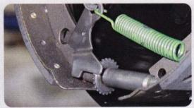
Self-adjusting brakes rarely self-adjust, which means drum brakes need to be adjusted periodically. Inspect and adjust drum brakes every 10,000 miles. This is a star wheel self-adjuster. If it works properly, it will advance the star wheel adjuster and shoes every time you back up and pump the brakes. This is why new hardware is vital whenever you perform a brake overhaul. Star wheel adjusters wear out with time and use.
