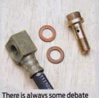
on what material to use at brake hose unions, but copper has always been the industry standard with aluminum as an acceptable alternative. Copper washers yield good crush qualities as do aluminum, which provides excellent sealing quality. It's suggested you only use them once and always install new versions during reassembly.
