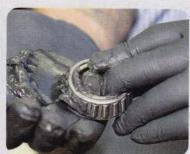
Always use a high-temperature wheel bearing grease even if you're building drum brakes. Use a good bearing packer or heavy massage work in the palm of your hand. Keep working the bearing in your palm until it's completely saturated with grease. Bearing failure happens when we fail to thoroughly pack the bearings or properly seat bearings on spindles.
