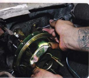
power brakes are old technology but still quite effective. When power boosters fail, you can expect high pedal effort or a pedal that won't return to rest. If the pedal won't return, you have a failed return spring. If there's high pedal effort, the diaphragm is damaged and there's a vacuum leak. In either case replace the power booster.
