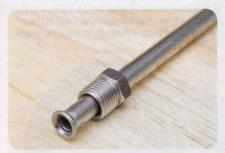
Brake lines are of double wall construction for the extreme pressures associated with hydraulic brakes. Galvanized steel lines get a double flare for unequalled sealing strength at each union. Stainless steel lines get a single flare via a stainless-specific flaring tool and collar.
