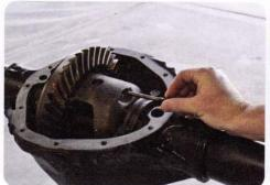
Once the cover is removed, locate and remove the bolt that holds the cross shaft in place, then remove the cross shaft. Now you can slide the axles toward the center of the differential and remove the C-clips.
