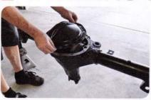
In order to swap from drum to disc brakes on the rearend, the axles must come out. Getting ready for the installation, we removed the diff cover. We already had the rearend removed, but this job can be done while it's still attached to your truck.
