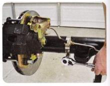
13 Tighten the clamp that holds the brake hose clamp in place, and then secure the brake hose to the caliper and hard line.
