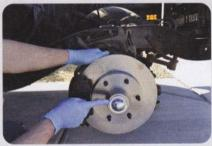
21 Cap off the rotor. You may need to tap it in place with a rubber mallet.
