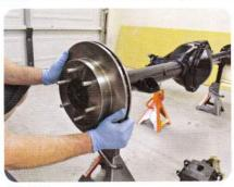
8 It's time to slide the rotor onto the axle. Make sure it's fully seated on the studs and axle.
