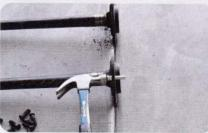
Once the axles are out, check to see if the new wheel studs are longer than the existing ones. If so, remove the old studs and replace them with the new versions. Hammer out the old studs and then hammer the new ones in their place.
