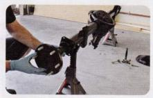
Slide the axles back into the housing. You may have to turn the axle a bit to line up the gears.
