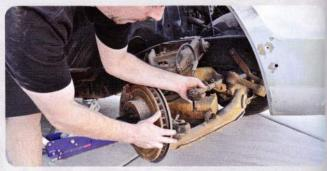
Disconnect the outer tie rods to replace the spindles. Remove the original spindle by taking off the castle nuts on the upper and lower ball joints. Take a minute to inspect the ball joints and replace them if necessary. Our lower ball joint is in terrible shape and must be replaced; however, since we will be replacing the arms and ball joints later, we decided to forego the additional cost right now.
