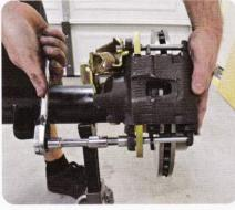
Install the caliper on the caliper bracket making sure the bleed screw is at the top. The CPP caliper slides in easily. We had no trouble with fitment at all and no need to shim the caliper. Tighten the bolts that hold the caliper in place, and make sure the rotor and axle can spin freely.
