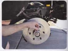
Tighten the spindle nut so that it's snug. Don't over tighten it! Spin the rotor forward to make sure the bearings are seated properly. Check the spindle nut. If it's still tight, move on, if not, tighten it again and repeat this step. Install the cotter pin to hold the nut in place.
