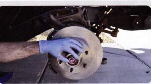
18 Slide the rotor onto the spindle. Install the outer bearing, washer and spindle nut.
