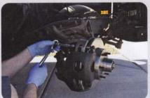
20 Install the front caliper assembly making sure the bleed screw is at the top. Again, our CPP calipers fit like a glove. Tighten the caliper bolts.
