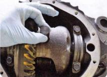
Slide the cross shaft back into place; this will hold tension on the C-clips. Reinstall the bolt that holds the cross shaft in place.
