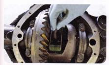
5 Install the C-clip into the axle. Be careful not to drop it into the differential. Then gently pull the axle back out away from the center of the housing. Repeat this on the other side.
