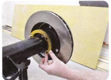
Using the hardware provided, install the spacer on the inside of the axle housing. Now install the caliper bracket and tighten them down with a washer, lock washer and nut.
