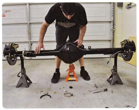
2 Attach the hard lines to the rearend and connect the brake hoses. Keep in mind that you will need to leave enough slack in the brake hoses to remove the caliper when it's time to replace the pads.
