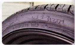
Remember to install the new emergency brake cable included with the kit. This was completed once the rearend was installed in our vehicle. Finally, you can install wheels and tires. We're running a set of 22-inch GM Transit wheels and 265/35R22 Toyo Proxes ST II tires. The Toyo Proxes ST II tires are directional, so pay attention when installing them on your vehicle.
