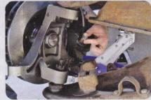
Install the brake lines using two crush washers, one on each side of the banjo fitting just like the rear. Tighten the brake lines. Next, install the outer tie rod end on the new CPP spindle.
