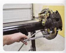
Install the brake hoses using a crush washer on each side of the banjo fitting. Don't tighten them, just snug them up on the rearend until the hard lines are in place and all of the brake line connections are made.
