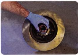
The new CPP 2-inch drop spindle was installed, and the upper and lower castle nuts on the ball joints were tightened. Pack the inner and outer wheel bearings with grease. Take your time with this step; it will prevent premature bearing replacement. Place the inner bearing in the backside of the rotor and then install the grease seal. You may need to tap it into place lightly.
