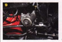
Three bolts hold the steering box to the framerail. One is inaccessible without removing the driver-side front bumper brace. Bumper alignment: The first step was to scratch a line to indicate where to remount the bumper.
