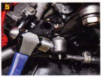
As shown in this image, removing the alternator and cast-iron alternator mounting bracket allowed for a straight shot to the stock Chevelle manual steering box.
