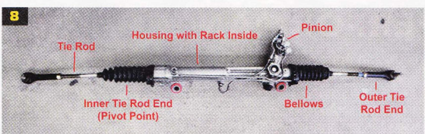
Here you can see how a power rack-and-pinion system works internally. Turning the steering wheel activates a rotary valve and sends high-pressure fluid to the appropriate side of the piston to assist in turning. – Drawing by Kris Horton.
