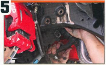
We were able to maneuver the box, with the pitman arm still attached, out of the Nova from the bottom. Depending on your headers you might need to loosen them up a bit to give a little extra maneuvering room.
