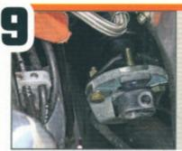
The coupler supplied by CPP was then fastened to the factory steering column. If you're very careful, you won't have to get your steering aligned due to your steering wheel being off-center.
