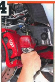
After disconnecting the pitman arm from the center link and removing the power steering lines, it was time to remove the old steering box. It's held to the frame by three %-inch bolts. After some persuasion the bolts broke free. It's heavy so gravity does most of the work here.
