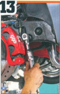
With the box in place we were then able to tighten the three bolts that hold the box to the frame.
