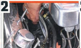
Using a line wrench, we broke loose and removed the high and low pressure power steering lines. We also disconnected the old rag joint from the steering column.
