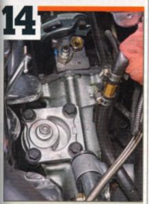
The last step was to reinstall our power steering lines. We then installed the pitman arm and secured it with the new nut and lock washer and secured it to the centerlink with a castle nut and new cotter pin. After double checking that all of the bolts were tight, we added some power steering fluid and took the Nova out for a test drive. The difference in steering feel was immense and it felt like we knocked 40 years off the car. Maybe that's because we did.
