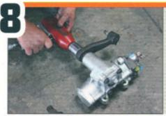
We then installed the pitman arm onto the new CPP power steering box. The easiest way is with an air impact gun as shown, but it can be done by hand with a bit more effort.
