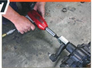
Next, we removed the old pitman arm from the stock gearbox. Sometimes it comes off with a few taps from a hammer, but ours had been on there a long time, so we broke out our trusty puller. If you don't have a puller they are cheap to buy or you can bum one off a buddy.
