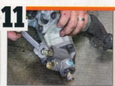
Due to the Nova's aftermarket hydraboost system, we installed this fitting so that we could use the preexisting -AN hose.
