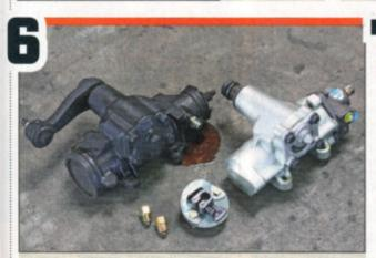
The new CPP 14:1 close-ratio box (PN 6774PSBS, \$399) is on the right next to the stocker. If you are hardcore into turning fast, CPP also offers the more aggressive 12.7:1 ratio, but for our Nova 14:1 is fast enough. We also picked up a new 1/4-inch 30-spline coupler (PN RJC730, \$49) and some adaptor fittings (PN 605ANFIF, \$25) so that the original power steering lines could mate to the new box.
