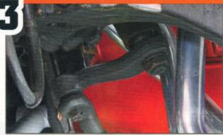
We then went under the car and disconnected the pitman arm from the centerlink. Ours came off pretty easily, but you might need to use a BFH (big freakin' hammer) or a pickle fork if it's a bit stubborn.
