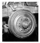
The front braking system looked exactly like the rear. a big drum. This system is not exactly up to today's standards for braking power and safety.
