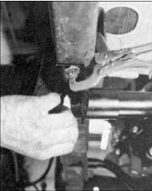
6. While they're under the truck, Alan and Ryan center the transmission between the frametrails. Sliding the crossmember side to side in the end collars makes it easy to adjust. They also mark the frame where it will need to be drilled for mounting bolts.
