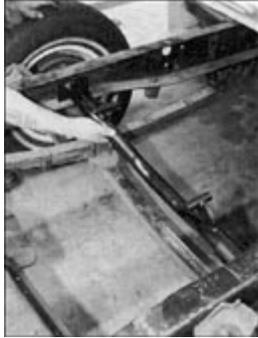
3. After sliding the end collars of the main tube, Alan positions the engine crossmember on the frame. Here nothing needs to be welded or bolted because the crossmember ends will rest on the frame's lower channel as the engine is positioned. Alan takes an educated guess on how far forward the crossmember will need to be (this will be adjusted as needed).
