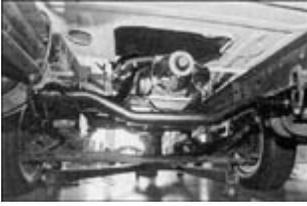
5. At this point you'll also want to mock the transmission cross member in place. Welding clamps or C-clamps work well to temporarily hold it in place.
