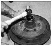
The job remained easy from here on out. The races were lined up in the hub, then started with a hammer by tapping around the perimeter until about halfway in. The old races were used to finish driving them into place.
