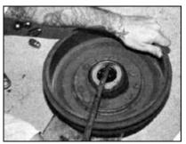
After the drum and hub are removed as one (at which time the front caged ball bearings and the inner race should fall loose), the rear retainer seal needs to be pried out. I found that removing the felt ring first allows the retainer to come out much easier.
