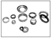
Once all the bearings and related parts were divorced from the hubs, I found that somewhere along the line someone had swapped certain bearings without changing the races, which could explain premature wear and excess slop. The outer left-side bearings actually had a plastic cage while all the others, varying in brands, were metal-caged.
