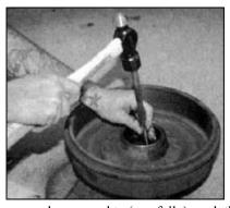
A medium punch was used to (carefully) work the old races out. In this case, each race came out with ease; others may experience more difficulty removing them. Beneath the hub I placed a small piece of tubing with an inner diameter large enough to allow the race to come out without interference.
