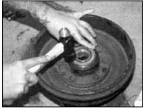
With the rear bearings all lubed up and packed with even more grease in the race, the rear retainer cover is carefully tapped in. CPP recommends using Loctite 640 "green" sleeve retainer to provide a secure adhesion of the seal.
