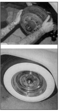
The tapered bearings slid onto the spindle nice and snug like, which told me I was in for a better ride as soon as I tightened-up the axle nut, slipped a cotter pin in place, then knocked the dust cover on. I will admit that I did experience quite a vibration after the initial road test, but come to find out, all four of my "shiny" chrome wheels were badly bent. Needless to say, the stock wheels were dug up, painted, and put back into service. Now, I've got a smoother ride than I ever expected.
