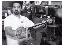
Test it to feel the movement of the shaft and also to see if there is any end movement. The shaft should spin smoothly and have no endplay.
