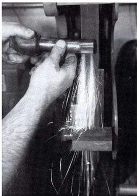
The spline end of the shaft is lightly sanded to make sure it is slightly under-sized. This will ensure that it fits the new bushings well. Now is the time to prep the shaft, not after you have installed the new roller, because you do not want any debris in the new needle bearings.
