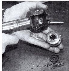
With the pin out, the roller is removed from the sector shaft. Notice the roller gear rides on needle bearings. Also, the washers will be used again.
