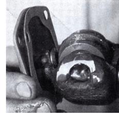
The washer slips into the notch in the end of the sector shaft, and the assembly is slid into place.
