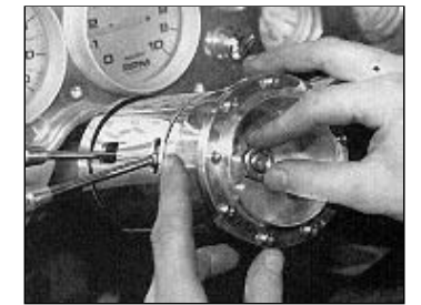
Most steering wheels will require an adapter such as this one from ididit. It's secured just like a factory steering wheel.
