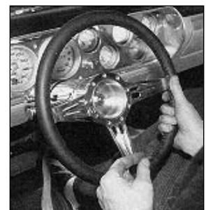
Most steering wheels will require an adapter such as this one from ididit. It's secured just like a factory steering wheel.
