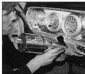
Using the factory rubber seal, the firewall plate was installed to the new column.
