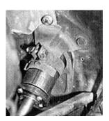
Back into the engine compartment, the firewall bracket and column clamp are reinstalled in their original locations. Make sure the upper flange of the firewall bracket slides UNDER the brake booster bracket not on top.
