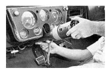
To install the new ididit tilt column, it is best to have someone hold the column in place from inside the engine compartment once it has been inserted through the firewall.
