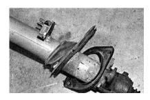
There's only one catch to the column swap. The factory firewall and dash rubber gaskets, as well as the firewall brace clamp, need to be removed. The rubber gaskets are available new from any 1967-71 parts dealer, but the metal brace is very difficult to find. To remove them from the old column, you can either take the stock column completely apart to get the shifter ear off, or you can cut it off. The bottom line is that these items, particularly the brace, have to be removed.
