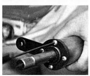
With these three parts in hand, install them on the ididit column by first removing the neutral safety switch, then removing the shifter arm that's bolted to the bottom of the column.
