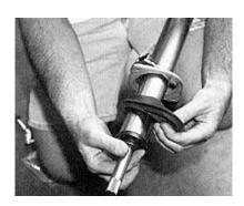
Next, slide the metal firevall brace and rubber gasket onto the column. Make sure they are installed facing the firewall. You won't want to have to redo this procedure once you've started installing the column.
