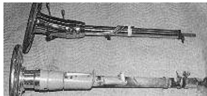
Here's a comparison of the old stock column and the new Ididit column.
