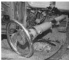
The column should now come completely loose.
