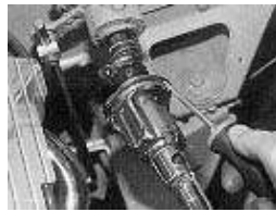
Loosen the metal boot by removing the metal safety clip.
