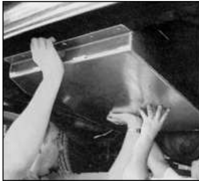
With the crossmember in place and the vent hose attached, the new tank is raised into position under the '57.
