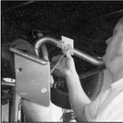
First we mount the new crossmember under the car.
