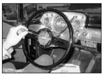
When installing the Lecarra Mark 10 wheel the first order is to install the wheel on the adapter.
