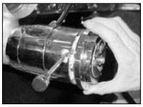
Next, install the adapter on the column. Slide it over the shaft in the column then bolt the adapter down.
