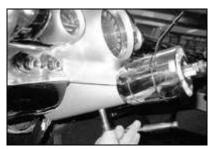
When it comes to mounting the new ididit column, there are a few brackets that hold it in place. Remove the old column and bolt up the new ididit column.
