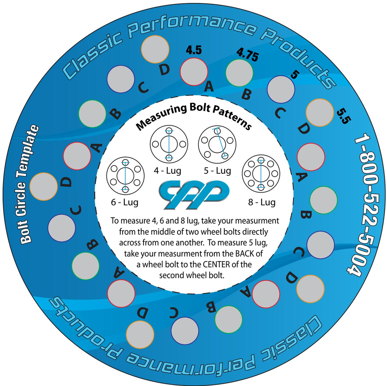
To use this Template. Cut out the center of the template, and place over hub. Line up bolts with the grey "bolt circles". The best fit will be your bolt pattern. For example, a 5 bolt hub that lines up with the 4 3/4" "bolt circles" (B) will be a 5 on 4 3/4" bolt pattern.
